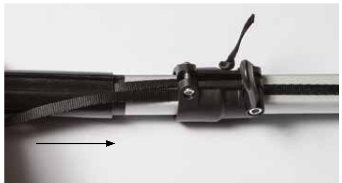
18. Align the black tube to the silver tube and slide up over plug.
