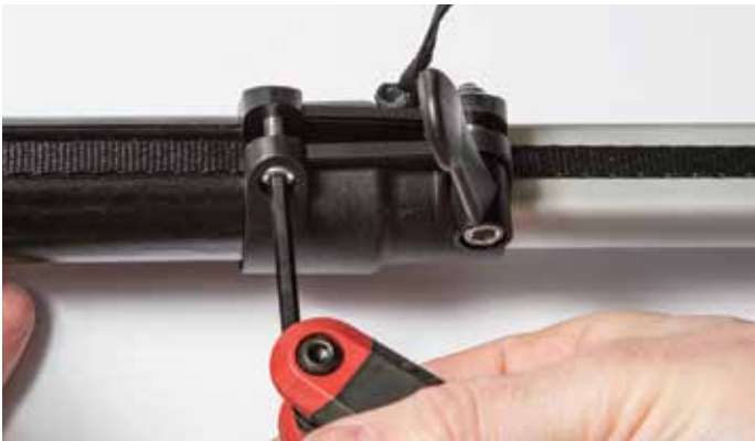
19. With the black tube in place, slide the clamp to the black tube.
