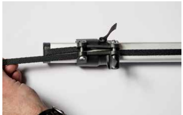
17. Once it is under the strap, pull snug so the strap does not twist.
