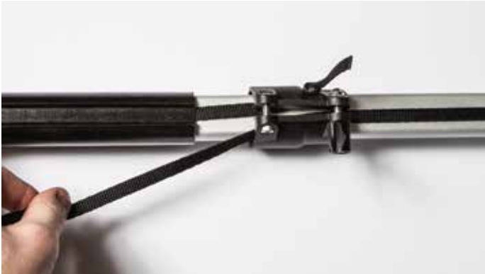
19. With the black tube in place, slide the clamp to the black tube.
