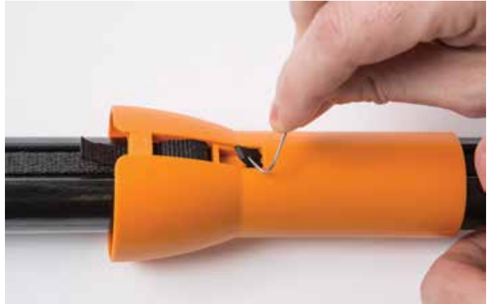
22. Use a paper clip or wire to pull the strap through the slot.
