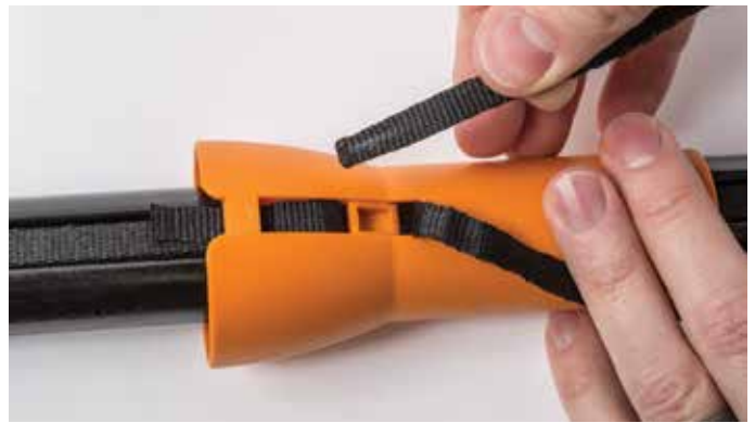
22. Use a paper clip or wire to pull the strap through the slot.
