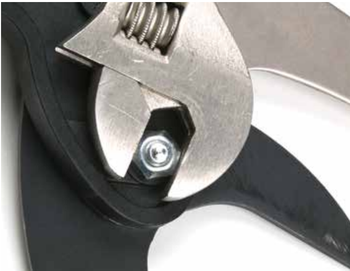
12. Actuate the tool using the orange handle. If the cutting blade will not fully open, use the crescent wrench to loosen the pivot nut/bolt until it does.
