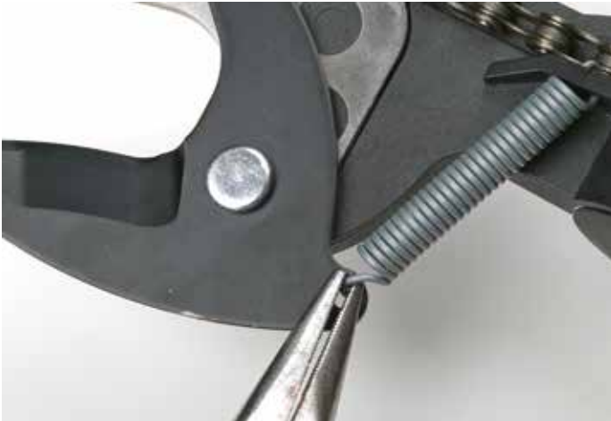
11. Use the needle nose pliers to attach the other end of the spring to the blade.
